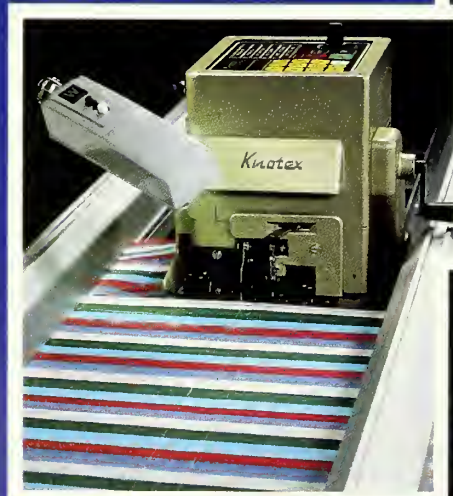
KNOTEX WARP TYING MACHINE has speeds up to 600 knots per minute.
